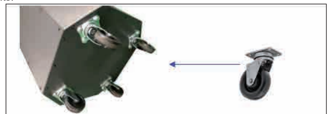
Step 31. Assemble the Octagon drum. Locate the drum base panel, (it does not matter which side faces inside), and secure the (4) casters using (16) 5/16" x 3/4" hex bolts, (32) 5/16" x 1" flat washers and (16) 5/16" hex nuts.
